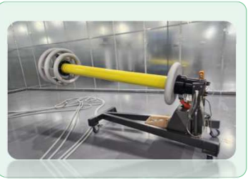
Cable Test Water Terminal
